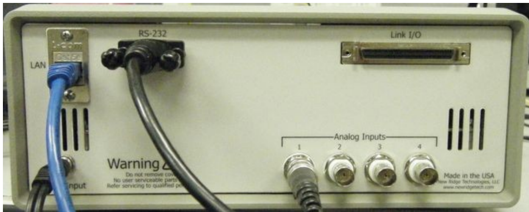
Figure 5: Rear of NRT-25xx ready for operation with a single analog input in stand-alone mode.
