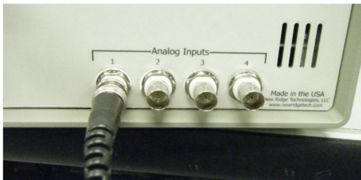
Figure 3: Analog connections (BNC) to the 4 ADC channels on the NRT-2500
