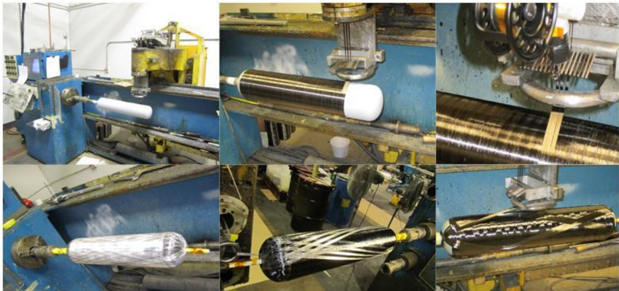
Figure 1. Compilation of photographs from flask manufacturing (clockwise from top left): Aluminum liner in filament winder, Application of carbon fiber/epoxy hoop layer, Application of optical fiber strain sensor (from reel above) simultaneously with carbon fiber/epoxy hoop layer, Application of helical carbon fiber/epoxy layer, Application of glass fiber/epoxy helical layer (for impact resistance), and Flask after completion of winding.
