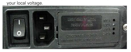
Figure 2. Power supply voltage selector, power cord connection, and on/off switch.
