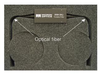
Figure 1 Tunable filter packed in special shipping case.
