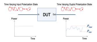
Figure 3. Measurement of component polarization-dependent loss (PDL)
