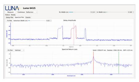
Figure 9. In the lower plot, the reflection spectrum of the second Bragg grating (selected and highlighted in red in the upper plot) is displayed
