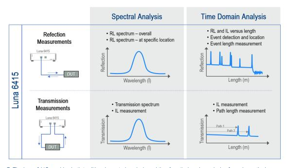
Figure 7. The Luna 6415 provides both traditional spectral analysis and time/length domain analysis of passive optical components; and is able to measure the loss of a DUT connected in reflection or in transmission
