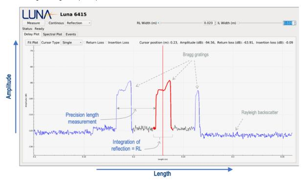
Figure 8. A scan of a Bragg gating string with a Luna 6415, connected in reflection, illustrates the high-resolution map of reflectance versus length, allowing high-precision measurement of RL, IL and path lengths
