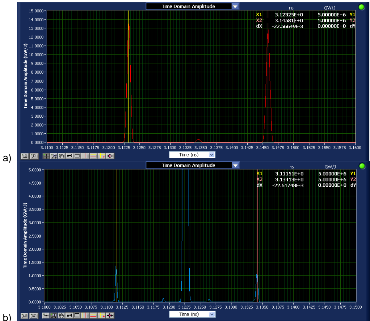
Figure 2. Time domain amplitude profiles of a) a FC-PC connector at the end of a 10 m PMF segment and b) a FRM with a 10 m PMF segment in the path to the OVA.
