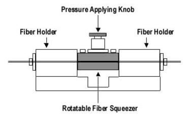
Figure 1 Diagram of manual polarization controller with functional parts labeled
