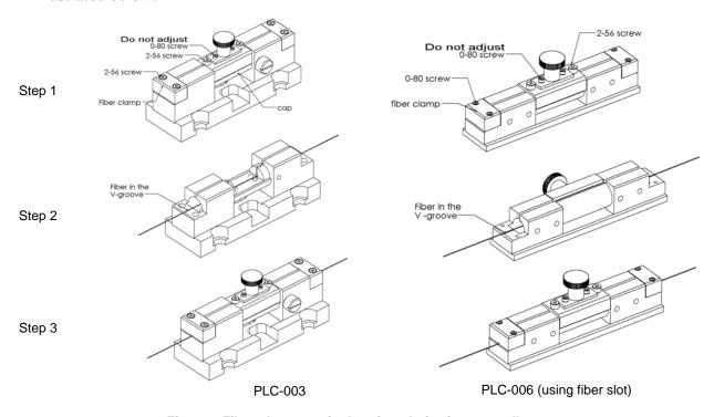
Figure 2 Fiber placement in drop-in polarization controllers
