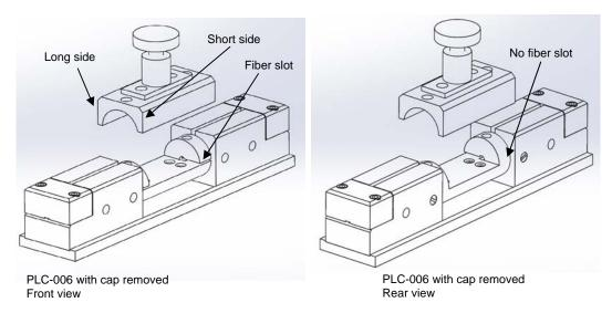
Figure 3 Center cap alignment for PLC-006
