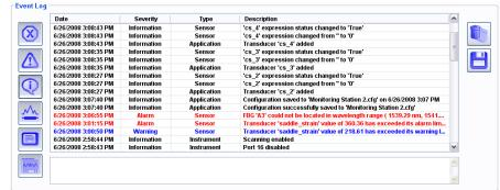
The image above shows the event log with multiple entries. To the left side of the chart are a series of filter controls that limit which events are shown in the table. To the right side are two controls used to delete or save the event log.
