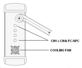
**CH1 (-CH4) FC/APC:** As many as four optical connectors can be found on the side panel of the si325module. Use only FC/APC jumpers to connect to the front panel FC/APC connectors.
