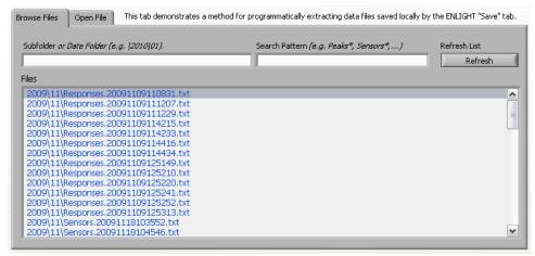
The fourth functional tab demonstrates a method for programmatically extracting data files saved locally by the ENLIGHT save tab. The #GET\_DATA\_ARCHIVE\_FILES command is used to list the files present on the user-specified subfolder and the #GET\_DATA\_ARCHIVE\_FILE command is used to extract and display the contents of the specified file.
