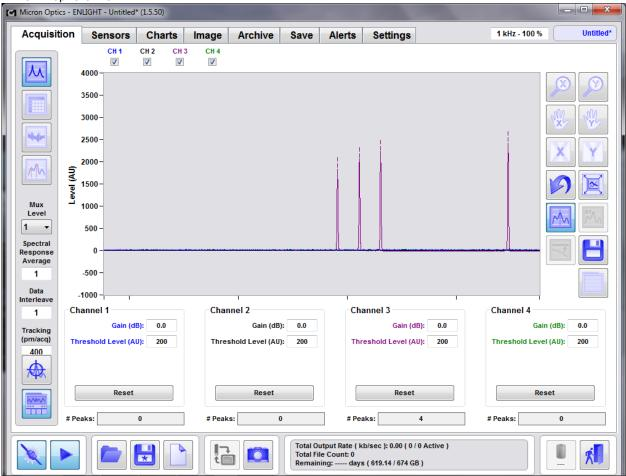
The preceding figure shows a full screen shot of MOI ENLIGHT with the Acquisition tab selected. Note that a large portion of the screenshot is filled with a tab control structure. This tab control dictates what features of the software are displayed based upon the tab selected. Note also that several controls and indicators are located outside of that tab structure. These features are visible on the GUI independent of the tab control state. The following section will detail those features.
