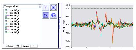
In the image above, ENLIGHT plots the Rate of Change for each of the nine os4100 relative temperature sensors and applies a positive limit of 1. An alarm will be triggered if any one of the nine sensors changes more than one degree C in a single acquisition.
