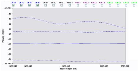
When the Mux Level is changed from 1 to 4, a interrogator core with a total number of four channels is multiplexed into 16 sub-channels. As is seen in the preceding figure, on the amplitude view of the Acquisition tab, the component sub-channels of each group share a common color. sub-channels are differentiated by line style. For each channel group (X = 1 - 4) = X.1: solid, X.2: long dash, X.3: short dash, X.4 dot-dash.
