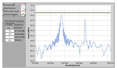
Case B: An additional 10 dB of insertion loss causes the spectrum to fall below the fixed Threshold value of -17.5 dBm.
