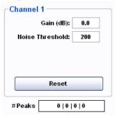
For x30 interrogator cores, peak detection is performed in channel hardware and during the actual laser scan. As such, the peak detection parameters are common among all of the sub-channels that make up a channel group, as shown in the figure above. Note that the resulting "# Peaks" indicator for the channel now reflects the two or four multiplexed sub-channels for that channel group, corresponding to the selected MUX level.
