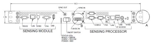
The ports for the sm230 Sensing Module are defined in the previous section. Addition of the Optional Internal Sensing Processor adds the following ports and connections.
