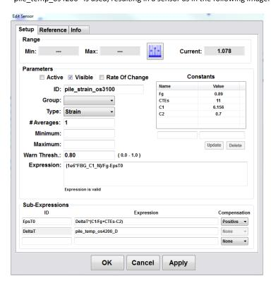
Note that the special DeltaT sub-expression references the absolute temperature sensor "pile\_temp\_os4200" with the "\_D" delta calculation shortcut, yielding a relative temperature quantity, as is needed for all DeltaT calculations. As with the os3600 example before it, EpsT0 uses DeltaT in a positively correlated compensation equation to normalize the thermal component of strain on the os3100 strain sensor.
