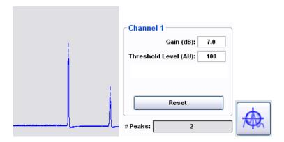
**Case II.** An additional peak is introduced to the system, yielding a greater number of detected peaks than tracked peaks.
