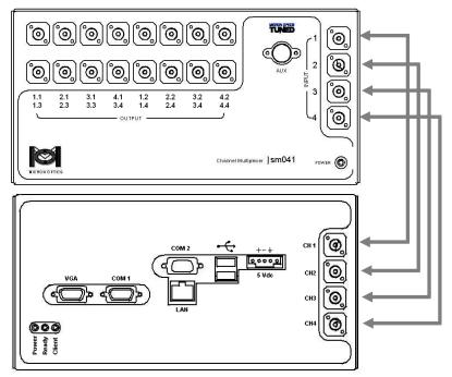
Diagram of sm041 optically connected to host instrument.
