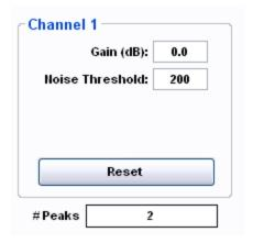
This group of controls is used to define the peak detection parameters for an x30 interrogator core, where peak detection is performed in the analog electronic circuitry of the interrogator. The resulting number of detected peaks for the channel is reported in the # Peaks indicator below the cluster.
