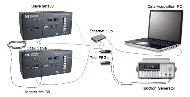
Hardware configuration for synchronized test measurement.
