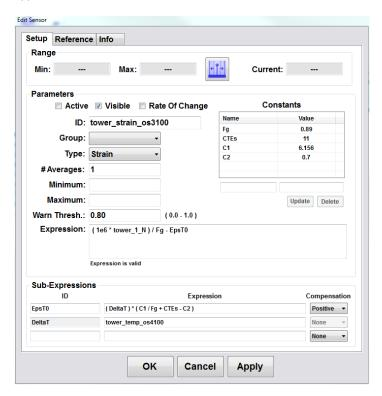
The strain calculation for the "tower\_strain\_os3100" takes the form of "strain = total strain – thermal component of strain".
