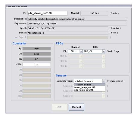
As with the previous two examples, most fields are automatically populated by the \*.mst file. For this sensor, the user chooses and ID, a substrate CTEs, and associates the strain measurement FBG (here FBG\_C1).
