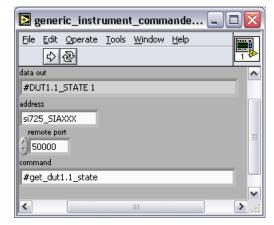
NOTE: Only port 1852 communications for the x30 and port 50000 communications for the x25 are supported via Ethernet Pass-through. For this reason, the web servers for the two interrogator cores are not available via Pass-through. Similarly, port 55000 internal peak detection commands are not supported for the x25 core via Pass-through, but port 50000 internal peak detection commands are.
