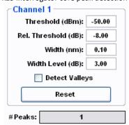
This cluster of controls is used to define the peak detection parameters for an x25 core, where peak detection is performed as a post processing operation on the full optical spectrum. The resulting number of detected peaks for the channel is displayed in the # Peaks indicator below the channel controls group.
