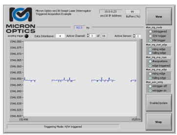
Hardware triggering configured for rising edge start, falling edge stop, with automatic retrigger off.
