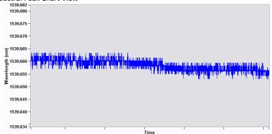
The Spectral Peak Chart View plots the wavelength value of one spectral peak as a function of time. A "Channel" control and "Peak #" control select the spectral peak to be plotted.
