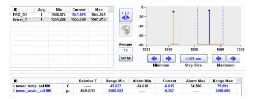
In the images above the limits for the "tower\_1" FBG have been dragged to set the range of the "tower\_strain\_os3100" sensor to a designed +/-2500 microstrain limit, over a --45 to 75 degrees C relative operating temperature range.
