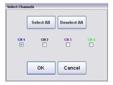
When a Create FBGs operation is initialized, a Select Channels popup window launches. A series of Boolean checkboxes offer the user control of which channels to select for automatic FBG bin creation, with the currently active channel pre-selected. "Select All" and "Deselect All" buttons offer a convenient means of mass channel selection. In the case that a multiplexer is employed in a configuration, the Select Channels window scales appropriately.
