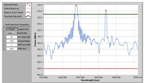
Case A: Starting point for peak detection explanation. Peak detection is enabled, peaks selected (as opposed to valleys), Rel. Thresh = -50, Threshold = -17.5, Width Level = 3dB, and Width = 0.03nm.
