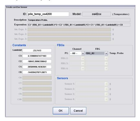
NOTE: os42xx and os43xx sensors require a large number of significant digits for the calibration expressions in order to yield the high absolute temperature accuracy that these sensors offer. Copy (control-c) and paste (control-v) operations are supported to ease data entry from other sensor data records.
