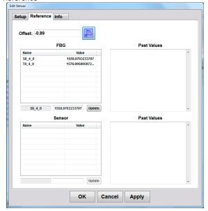
The Reference tab on the Edit Sensor window displays the composition of a sensor referencing multiple FBG or sensor elements.
