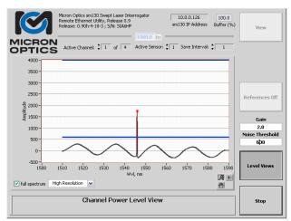
Use of the Noise Threshold Level control to eliminate false sensor detection
