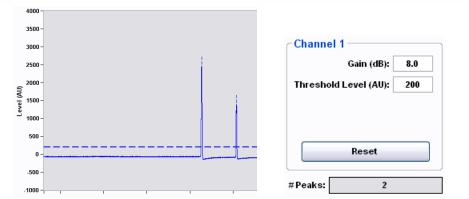
Note the transient dashed line that appears for 1 second to indicate that the Noise Threshold value is changed. This indicator also appears briefly when the Gain control is changed. Dashed lines also indicate threshold settings for x25 interrogator cores.
