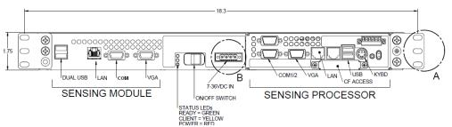
The ports for the sm225 Sensing Module are defined in the previous section. Addition of the Optional Internal Sensing Processor adds the following ports and connections.
