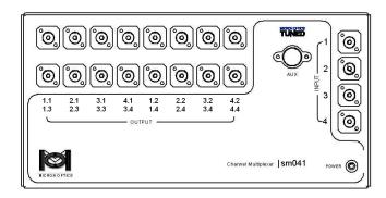
**POWER LED:** This red indicator confirms that power has been supplied to the module. A switch-type sm041 module (e.g. sm041-416) requires no separate power supply of its own, as all power and control for the multiplexer are supplied from the host interrogator module via the AUX port. A coupler-type sm041 module (e.g. sm041-016) is passive and requires only optical connectors. See INPUT and OUTPUT below.
