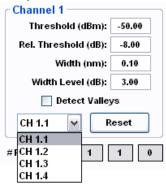
For x25 interrogator cores, peak detection is performed as a post processing step on acquired spectrum. As such, the peak detection parameters can be individually specified for sub-channels, as shown in the figure above.
