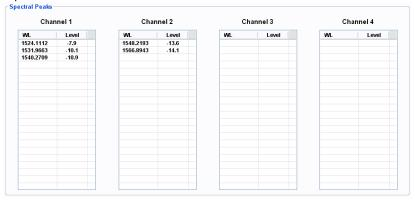
The Spectral Peaks table displays the wavelength and amplitude level information for all of the spectral peaks detected on a per-channel basis. x25 interrogator cores report level in dBm and x30 interrogator cores report level in arbitrary units.
