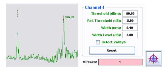
Following the example further, it is seen that the first spectral peak on channel 4 (which corresponds to FBG "FBG\_D1") has fallen below the Rel. Threshold Level of -8 dB. With this information, the user can either seek to correct the root cause of the attenuation or change the peak detection parameters in order to re-enable detection of the missing spectral peak.
