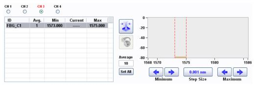
The absence of the grating is indicated by the red bin limits and channels 3 label, but sensors can still be created from the FBG C1 reference.
