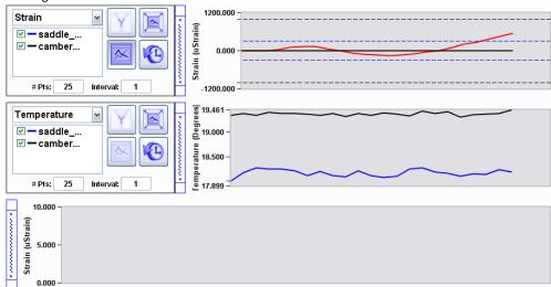
When a sensor goes into warning or alarm condition, the color of that sensor plot on the chart turns from its predefined color to either yellow or red, respectively. In the above figure, it can be seen that the "saddle\_strain" sensor has exceeding its maximum limit value and is thus in an alarm state. As such, the color of its trace has turned from blue to red.
