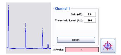
The preceding graphic shows a condition where a spurious peak has been introduced to the sensor system, and has been detected by the x30 interrogator. In this example, the three tracked and detected peaks are indicated by the blue vertical lines. The red-highlighted "# Peaks" indicator shows that a total of four peaks have been detected, though only three have been tracked. This fourth peak will not be included in any subsequent FBG or sensor definitions unless included among the tracked peaks.
