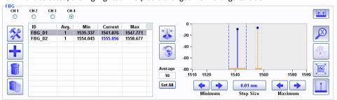
In the image above, the FBG "FBG\_D1" has been selected, and its image has been highlighted on the graph in blue to aid with visual association. Also note that the FBG bin limits for all other FBG entries have been grayed out, further highlighting the selected FBG and its bin controls.
