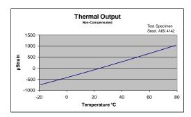
There are several methods of determining the thermal output of a gage. Once the thermal output is known, the mechanically induced strain can easily be calculated by subtracting the thermal output from the strain measured by the active gage as follows: (Note the introduction of a scaling factor that more conveniently expresses strain in units of  $\mu$ m/m)
