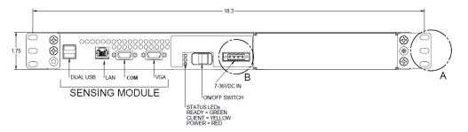
**POWER LED:** This red indicator confirms that power has been supplied to the module.
