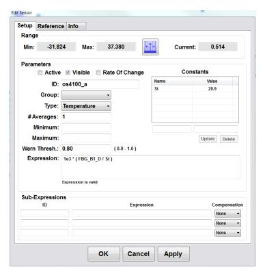
This sensor will now report its derivative, calculated by a five point Savitzky-Golay convolution, for plotting and alarm purposes.
