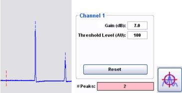
There are several ways to rectify the alarm condition caused by a mismatch of detected and tracked peaks.
