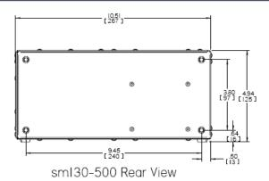
**MOUNTING HOLES.** These threaded holes on the rear of the sm130 allow for direct mounting of the module.
