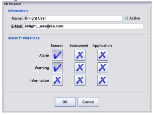
The preceding figure shows the data entry form used to configure the attributes of a selected notification recipient. In addition to the Information parameters already discussed in the previous section, there are controls to filter the type and severity of information that will be considered for triggering a notification event.
