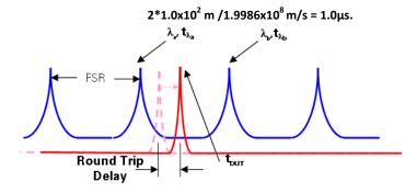
Timing diagram for reference/DUT calibration with round trip delay.
