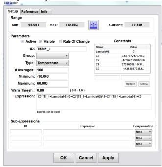
This Edit Sensor dialog is a data entry form used to set/modify the attributes for the selected sensor element. This form is launched by use of the "Add Sensor" and "Edit Sensor" buttons, as well as a double click event on one of the sensor entries on the table, in the case of a desktop deployment.
