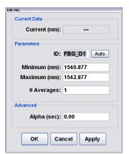
Note that the default wavelength bin width of 2nm has been applied to FBG\_D1.
