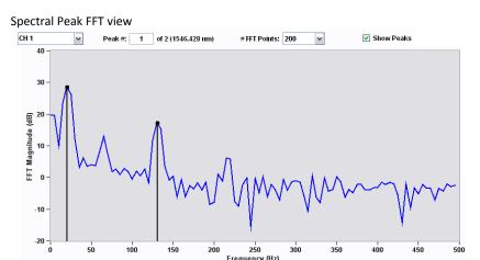
The Spectral Peak FFT View plots the frequency response of one spectral peak as measured by an x30 interrogator core. A "Channel" control and "Peak #" control select the spectral peak whose frequency response will be plotted. The "# FFT points" control selects how many sequential data points are used to calculate the FFT. The "Show Peaks" control overlays indicators of detected FFT feature in the Fourier spectrum.
