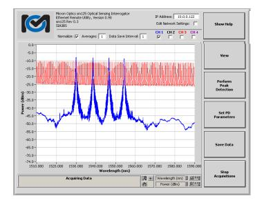
The preceding figure shows the sm125 measuring a mixed collection of FBG and Fabry-Perot Sensors. The FBG sensors can be seen on Channel 1 represented by the blue trace, and selected by the blue-labeled checkbox control "CH 1." The FP sensor can be seen on Channel 3, represented by the red trace and selected by the red-labeled checkbox control "CH 3."
