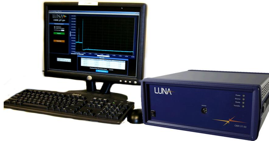
Figure 1-1 OBR measurement system. The OBR is a high resolution reflectometer designed for interrogating optical components and modules.
