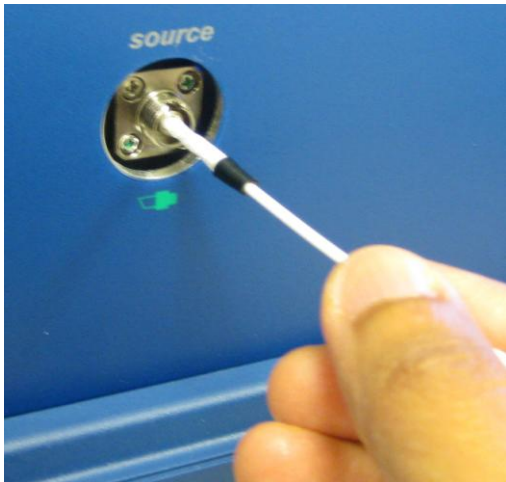
Figure 7-1 Remove the protective cap. Gently insert supplied mini swab, rotate in one direction, then remove.
