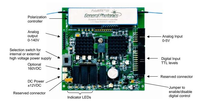
Figure 1 Top view of PCD-M02 (MPD-001 board with integrated PolaRITE III polarization controller) with principal electrical connectors labeled.
