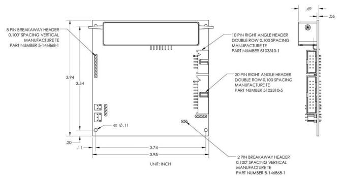
Figure 4 Dimensions of MPD-001/PCD-M02
