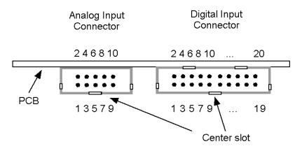
Figure 3 Analog and digital input connector configurations.
