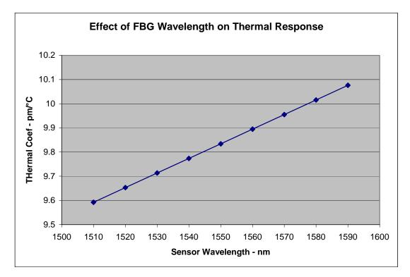
This variation can be approximated linearly relative to the sensor wavelength and is shown below.
