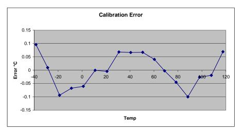
Figure 3 – Typical Error from 3<sup>rd</sup> order Polynomial Curve Fit
