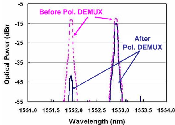
Fig. 3. Concept proof using two static wavelength channels with different power levels: here the power difference is  $\sim 0.5$ -dB (before Pol. DEMUX), and an ER of  $\sim 28$  dB is achieved with the proposed polarization demultiplexing scheme (after Pol. DEMUX).  $>35$ -dB ER is possible as the power difference increases.
