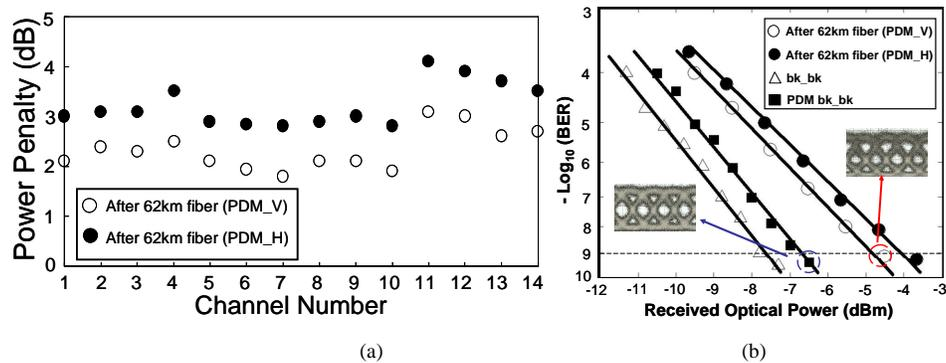
Fig. 6. Transmission results (a) Power penalties of both polarization channels (PDM\_V and PDM\_H) for all 14 wavelength channels compared to the back-to-back PDM system sensitivity measured at  $10^{-9}$  BER. (b) Typical BER curves of one wavelength channel with eye diagrams inserted: bk\_bk (back-to-back case without PDM transmitter); PDM bk\_bk (back-to-back case with PDM transmitter).
