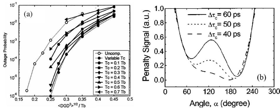
Fig. 17. Benefits to first-order PMD compensation using tunable DGD elements. (a) Comparison of outage probability with fixed and tunable DGDs in 33% duty cycle OOK-RZ transmission systems ( $T_c$ : delay line length;  $T_b$ : bit period) (from [50]). (b) Diagram illustrating the existence of local minimums during tracking using fixed DGD compensator ( $\alpha$  is the angle between the fiber and compensator PMD vectors) (from [51]).
