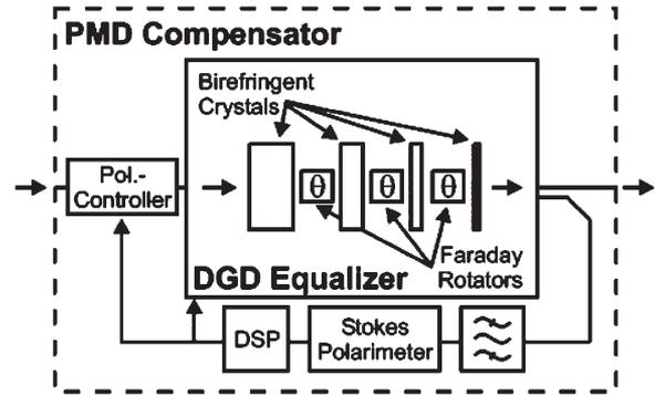
Fig. 18. First-order PMD compensator based on birefringent crystals, MO polarization rotators, a LiNbO<sub>3</sub> polarization controller, a bandpass filter, a polarimeter, and a digital signal processor (DSP) (from [52]).
