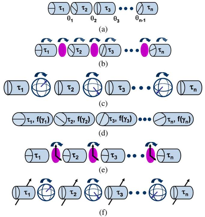
Fig. 4. Models of PMD emulators. (a) Fixed. (b) Rotator. (c) Scattering. (d) Phase. (e) Rotator + switch. (f) Tunable. (Color version available online at <http://ieeexplore.ieee.org>.)
