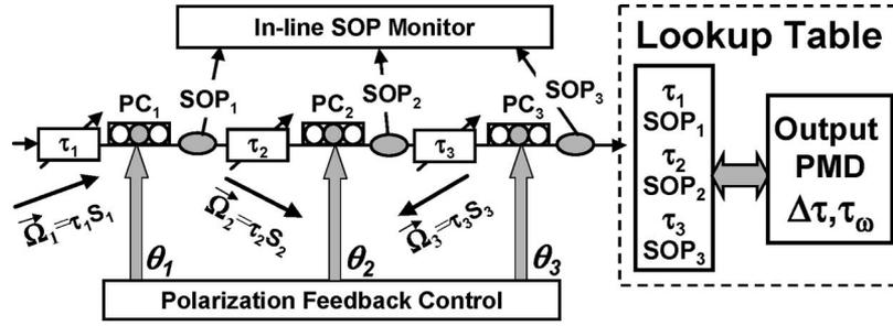
Fig. 9. Emulator setup incorporating simple in-line polarimeters with automatic feedback to control the SOP between sections to enable the generation of a lookup table of input DGD and SOP values versus output DGD ( $\Delta\tau$ ) and SOPMD ( $\tau_\omega$ ) values.
