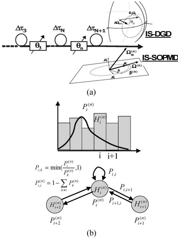
Fig. 10. (a) IS method using preferential alignment of PMD vectors. (b) MCC procedure.
