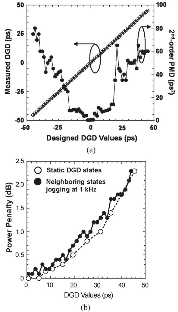
Fig. 7. Typical characteristics of the programmable DGD element. (a) Measured DGD and SOPMD as a function of the designed DGD values. (b) Dynamic performance in a 10-Gb/s NRZ system: Power penalties measured using an optical preamplified receiver of static DGD states (open circles) and dynamic switching (“jogging”) between neighboring states at 1 kHz (solid circles).
