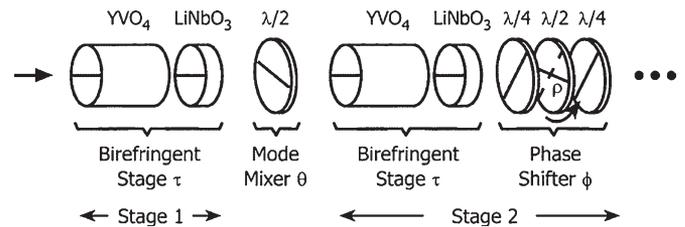
Fig. 2. First two stages of a four-stage coherent programmable PMD source (ECHO) (from [16]).
