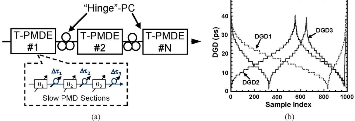
Fig. 15. (a) Conceptual diagram of a “hinge” emulator using multiple T-PMDE containing programmable DGD elements (T-PMDE) with slow PMD dynamics. (b) To realize the slow PMD dynamics for a single tunable emulator [T-PMDE shown in 16(a)], the DGD evolution is reorganized for three DGD elements with slow variations from sample to sample ( $\sim 1000$  samples). (Color version available online at <http://ieeexplore.ieee.org>.)
