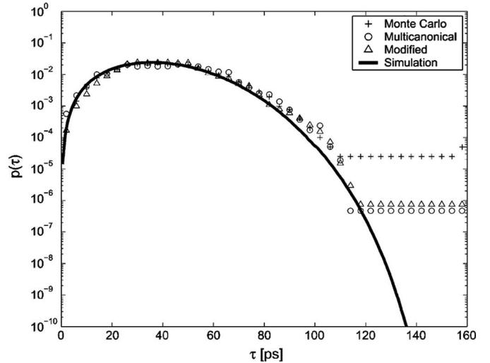
Fig. 11. Experimental comparison of MCC sampling techniques with a conventional Monte Carlo method using a 30-section PMD emulator (from [43]).
