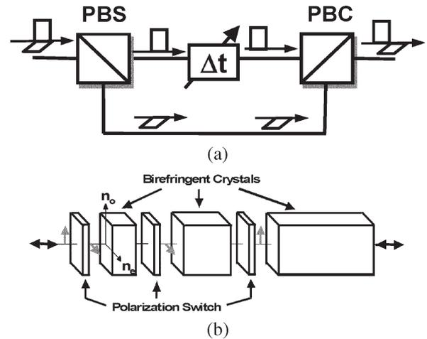
Fig. 1. (a) Tunable DGD emulator based on bulky optical components (PBS: polarization beam splitter; PBC: polarization beam combiner). (b) Conceptual diagram of a programmable DGD element using binary polarization switches and birefringent crystals.
