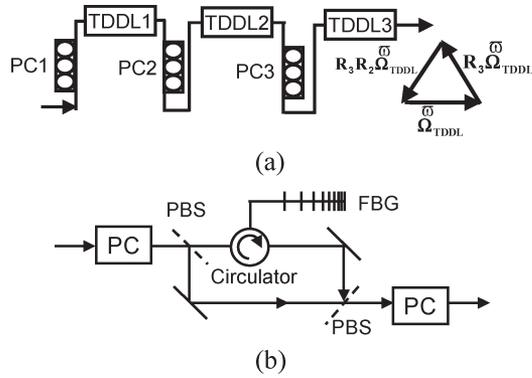
Fig. 3. (a) Interferometrically stable three-section higher-order PMD emulator (TDDL: tunable differential-delay line) (after [20]). (b) Isolated higher order PMD emulator using fiber Bragg gratings (after [8]).
