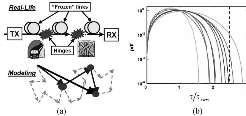
Fig. 14. (a) “Hinge” model in which most of the spans remain frozen over weeks, or months, and several dynamic “hinges” exist that are responsible for any significant changes in the PMD. (b) Sample DGD pdfs for ten statistically independent channels in a six-segment system indicating that most of the channels have a zero probability of exceeding  $2.5 \tau_{rms}$  (from [47]).
