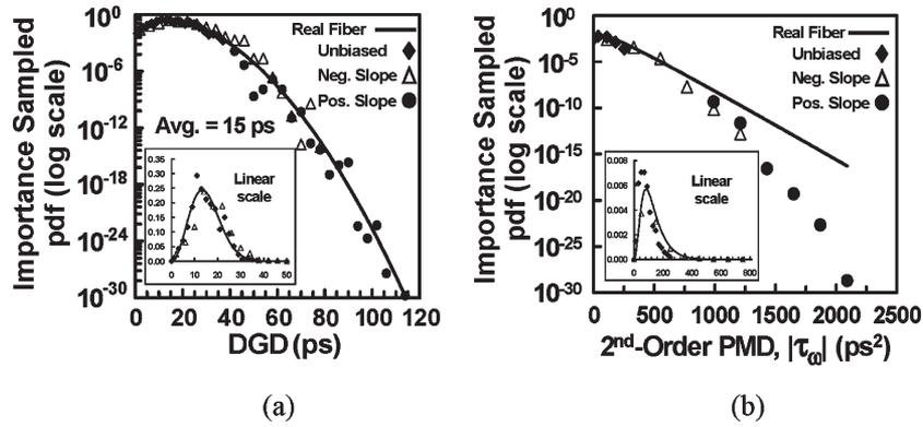
Fig. 13. Experimental results using multiple IS to provide a better coverage through the entire sample space. Three DGD distributions applied to each section (840 samples/each). (a) Resulting DGD distribution showing that each pdf generates samples in different regions to cover the entire Maxwellian, and (b) resulting SOPMD pdf. The insets show the pdfs on a linear scale.
