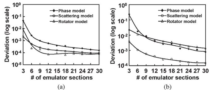
Fig. 6. Comparison of three emulator models: the rotator, scattering, and phase models [15]. The plot shows the deviation from the statistical distributions expected from a real fiber with the same average DGD versus the number of emulator sections. (a) DGD deviation from Maxwellian. (b) SOPMD magnitude deviation from theory.
