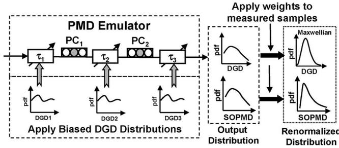
Fig. 12. Conceptual diagram of applying the IS method to the T-PMDE, which is accomplished by applying a biased DGD distribution to each section and then appropriately weighting the results to obtain the desired pdf.
