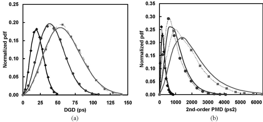
Fig. 5. Simulation results of a “rotator + switch” PMD emulator, as proposed in [26]. (a) DGD distributions with  $\langle \Delta\tau \rangle = 21, 43,$  and  $60$  ps. (b) Corresponding SOPMD distributions with  $\langle \Delta\tau_\omega \rangle = 215, 937,$  and  $1705$  ps<sup>2</sup>, respectively. All of the distributions were obtained from the same emulator.
