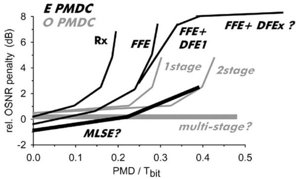
Fig. 19. Estimated penalty versus PMD-limits of electronic (dark lines, E-PMDC) and optic (shaded lines, O-PMDC) PMD compensators (from [67]). (FFE: feed-forward equalizer; DFE: decision feedback equalizer; and MLSE: maximum likelihood sequence estimation).
