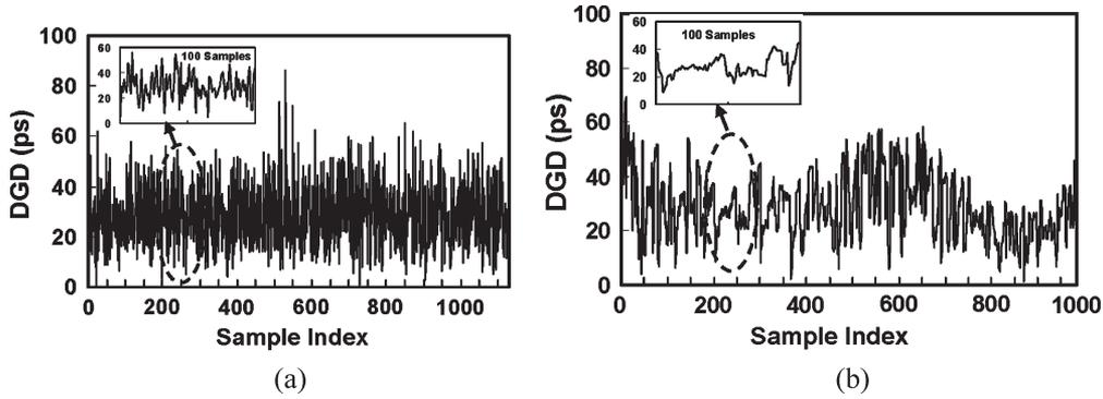
Fig. 16. Comparison of generated PMD dynamics (negligible distortion on the overall PMD distribution). (a) Previous approach using random DGD and random polarization coupling as described in Section III. (b) Slow PMD dynamics approach.
