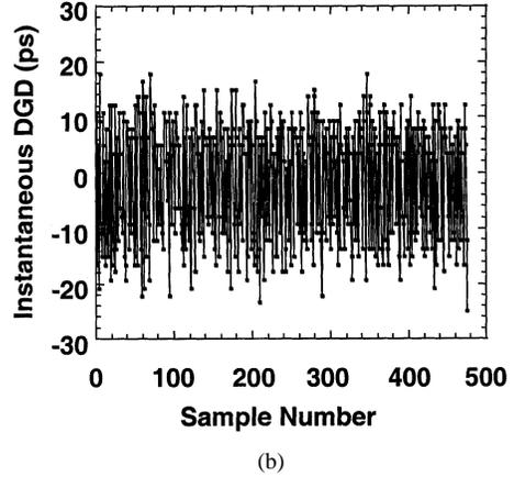
Fig. 6. Repeatable DGD generation is used to generate dynamic first-order PMD distribution with tunable average values. (a) First-order PMD distribution of 500 samples with an average DGD of 10 ps. (b) Instantaneous DGD values of the samples.
