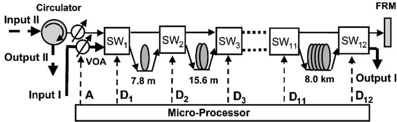
Fig. 1. Configuration of the programmable delay generator (ODG), single-pass (input I and output I) and double-pass (input II and output II);  $SW_i$ , MEMs-based optical switches; FRM, Faraday rotator mirror; VOA, Variable optical attenuator.
