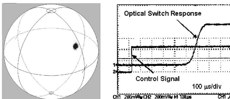
Fig. 3. (a) Polarization stability of the double-path configuration with external polarization perturbation; (b) measurement result of the response time for the ODG:  $<1$  ms ( $\sim 700 \mu\text{s}$ ).
