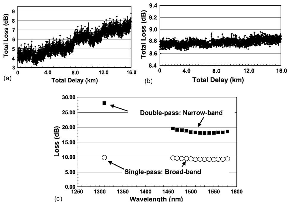
Fig. 2. (a), (b) Insertion loss variation at different delay settings (2048 logic states for the single-pass configuration at 1550 nm): (a) without automatic power balancing (b) using the VOA to automatically control the overall loss, thus the total variation  $<0.3$  dB. (c) Insertion loss variations of the ODG at different wavelengths (single pass at  $40 \mu\text{s}$  and double pass at  $80 \mu\text{s}$ ).
