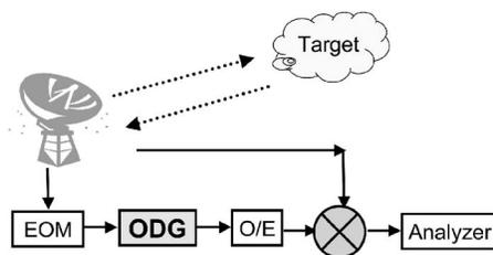
Fig. 5. Illustration of a rf ranging or calibration system utilizing the ODG platform. EOM, electro-optic modulator.
