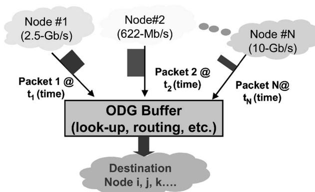
Fig. 4. Using ODG as a tunable optical buffer for a dynamic packet-switching network.
